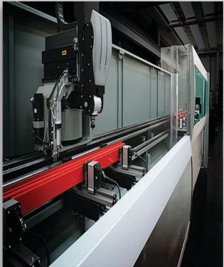
**4-axis** CNC machining center with moving gantry structure. Designed for drilling, milling, thread cutting and cutting at angle any from 0° to 180° on bars or workpieces of aluminium, PVC, light alloys in general and steel.
